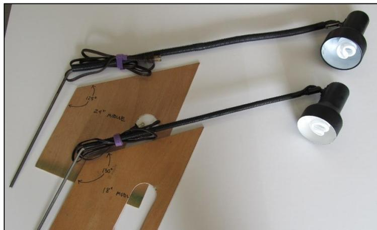
18. Insert the support rod to the neck. Wrap the flex tubing (the flex tubing is split to make this easy) around the rod and extension cord and secure the top of the rod and extension cord with black tape. Use small black zip ties to secure the rod, extension cord and the flex tubing together.
